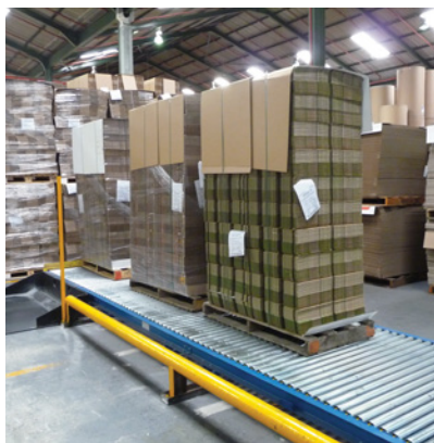
Accumulation Driven Roller Conveyors (Stacks and Pallets)
