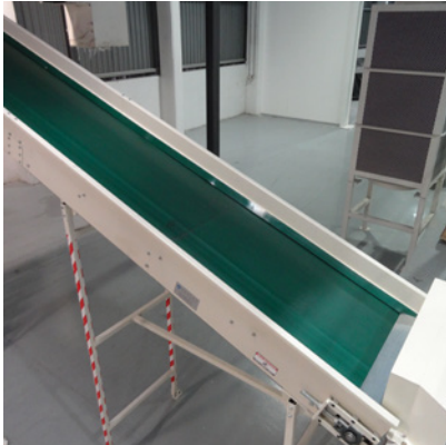
Waste Belt Conveyors
