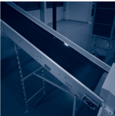
Waste Belt Conveyors
